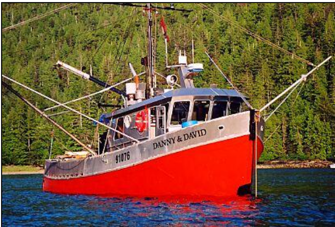
Plate 9: Converted for use as a packer in the seafood harvesting industry, the 18-m Danny & David proved to be the ideal vessel for the trip to Bowie Seamount. Its fish-hold was flooded to provide a means of transporting live specimens back to Vancouver.
